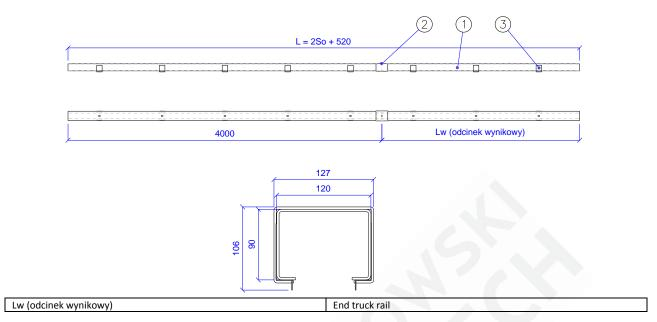
Fig. 4 – MARC–P(1)60-01.02.00 [Truck rail assembly]
