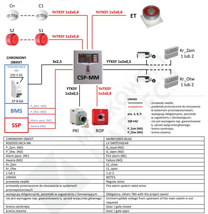
Fig. 13 - MARC-P1 control system with electromagnetic holder
