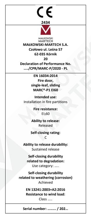
Fig. 15 – Specimen of the nameplate of the sliding fire door (ref. EN 16034:2014-11)
