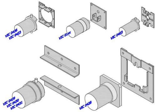
Fig. 9 – ISOiK-Ok60-01.09 [handles for individual internal drives]
