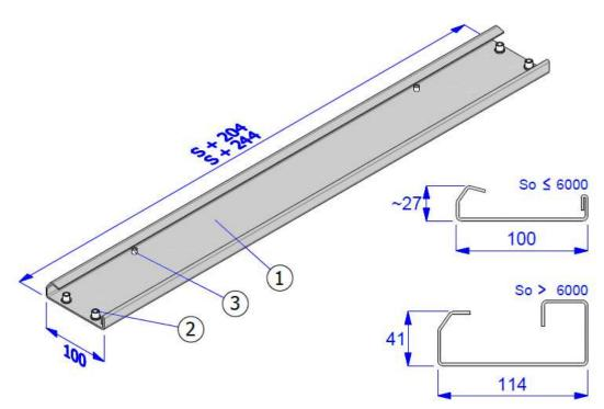
**Fig. 11 – ISOiK-Ok60-01.11 [push bar]** 1 – Bar profile, 2 – Rivet nut, M6, 3 – Rivet nut, M5
