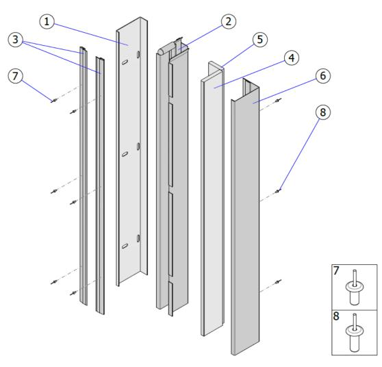
Fig. 21 – ISOiK-Ok60-01.21 [guide rail – wall-mounted version]
