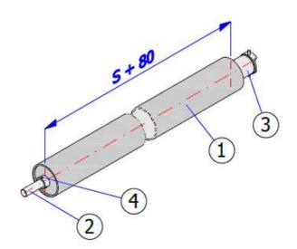
Fig. 5 – ISOiK-Ok60-01.05 [winding shaft with internal drive] 1 – Shaft tube, 2 – Journal, 3 – VIC type internal drive, 4 – Pressure screw
