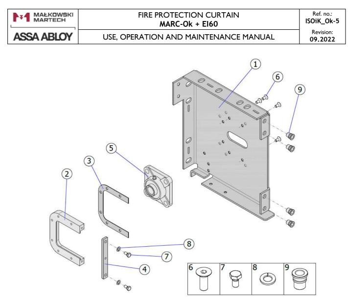
Fig. 24 – ISOiK-Ok60-01.24 [shaft bracket – passive side]
