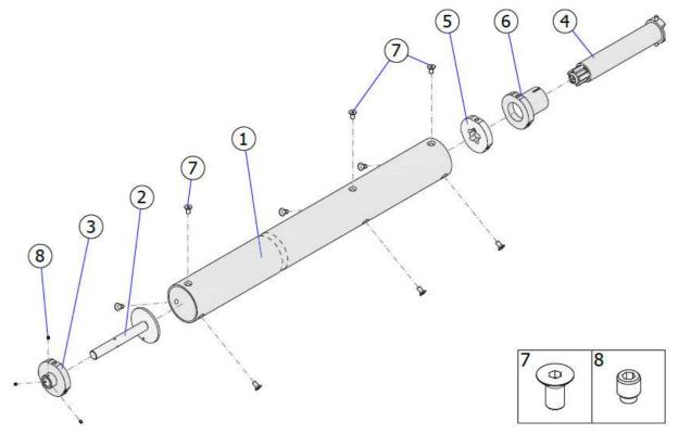
Fig. 19 – ISOiK-Ok60-01.19 [winding shaft with internal drive]
