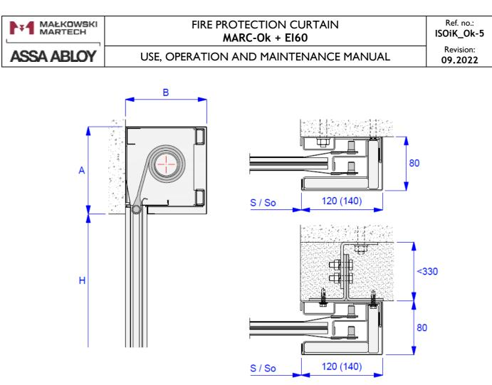
Fig. 3 – ISOiK-Ok60-01.03 MARC-Ok + EI60 fire protection curtain door – wall-mounted S – clear travel width, So – gate opening / building wall opening width H – clear travel height, Ho – gate opening / building wall opening height
