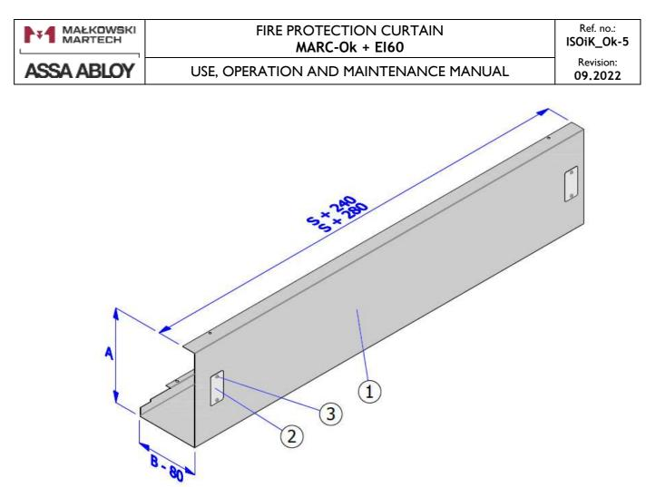
**Fig. 13 – ISOiK-Ok60-01.13 [front guard]** 1 – Guard profile, 2 – Inspection hole cap
