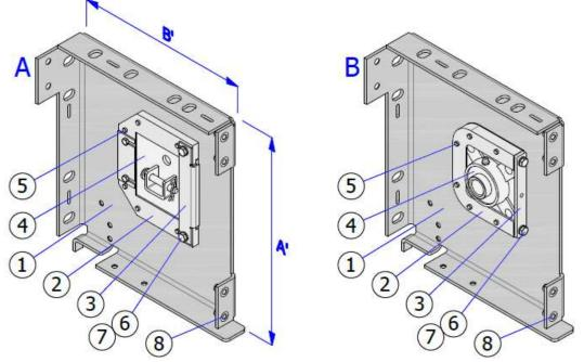
Fig. 8 – ISOiK-Ok60-01.08 [Shaft bracket, A – drive side, B – passive side] 1 – Bracket body, 2 – Drive / bearing bracket, 3 – Drive / bearing lock, 4 – Drive holder / bearing, 5 – M8 x 25 screw, 6 – M6 x 12(14) screw, 7 – Spring washer, 6.1, 8 – Rivet nut, M6
