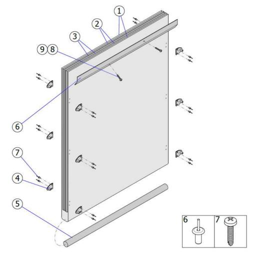
Fig. 20 – ISOiK-Ok60-01.20 [door sheet]
