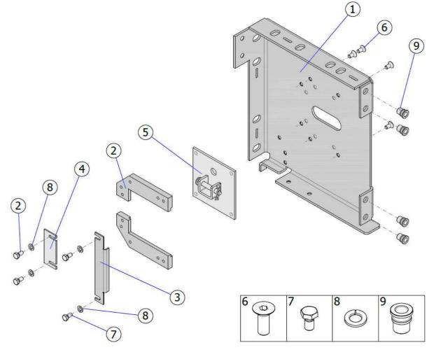
Fig. 23 – ISOiK-Ok60-01.23 [shaft bracket – drive side]
