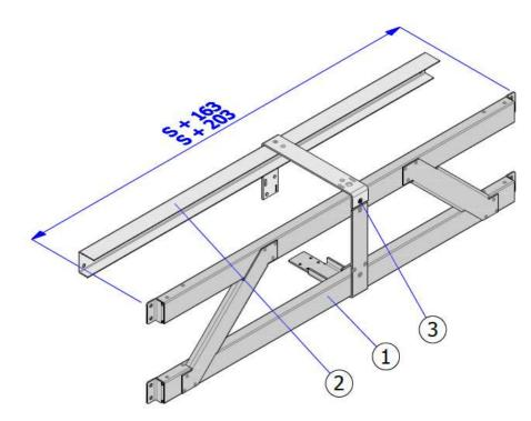
**Fig. 10 – ISOiK-Ok60-01.10 [structural lattice with wall-mounted channel section]** 1 – Lattice structure, 2 – Wall-mounted channel section, 3 – Sheet-metal screw
