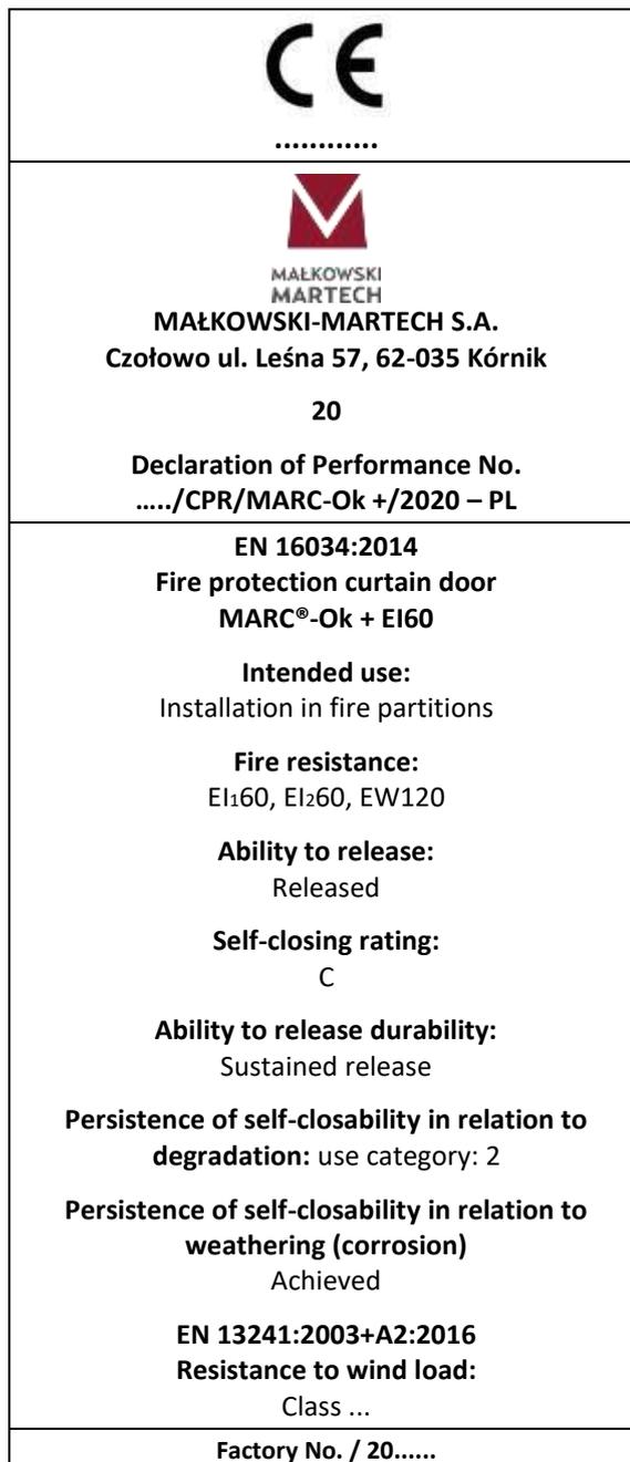
**Figure 31 – Examples of MARC-Ok + EI60 fire protection curtain door nameplate according to EN 16034:2014-11)**
